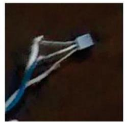
Fig2. Temperature Sensor (LM35)
